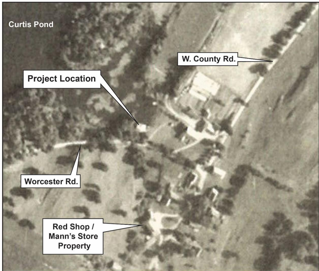
Figure 31. Detail of a 1942 aerial photograph showing the project location and surrounding area (Air Mapping Corp. 1942). The appearance of the dam in this photo suggests that the spillway may have been blocked off at this time, raising the impoundment and causing nearly the whole structure to become a primary spillway; it is also possible that the boathouse mentioned in the records appears in the image. Also note the “Red Shop” complex before the fire of 1947 and its position directly along the stream.
